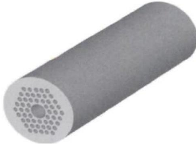
Fig. 1.3. A schematic drawing of an example of a photonic crystal fiber
