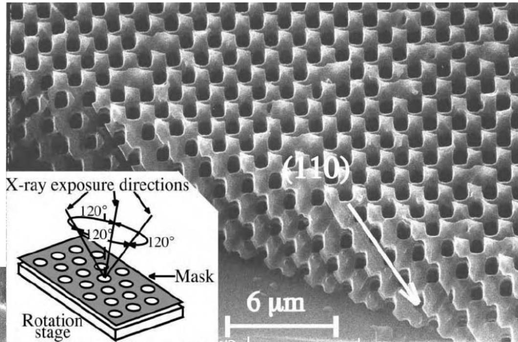
**Figure 8-21** Yablonovite is formed by **drilling holes** into a dielectric at three precise angles, and results in a diamond - like structure. The holes can be created by exposure to **X-rays** through a mask
