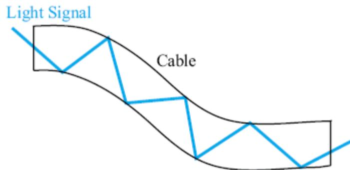
➤ **TIR** fundamental Principle Operation
