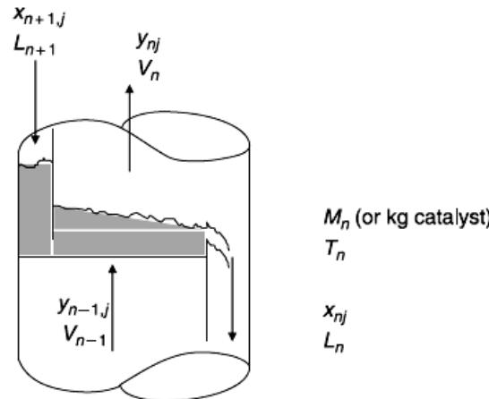
$$R_n = M_n (k_{F(T_n)} X_{nA} X_{nB} - k_{B(T_n)} X_{nC} X_{nD})$$
