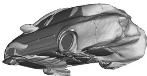
Fig. 14.24. Isocontours of total pressure. Courtesy of Renault-Aerodynamic Department.
