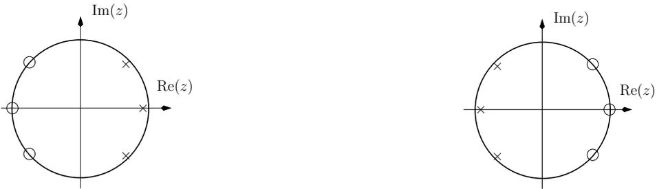
Figure 5.16: Pole and zero locations of a low pass filter (left) and of a high pass filter (right)
