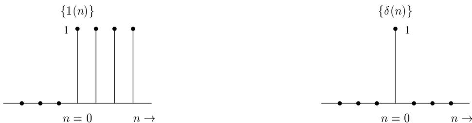
Figure 3.6: Unit step (left) and unit impulse (right) signals
