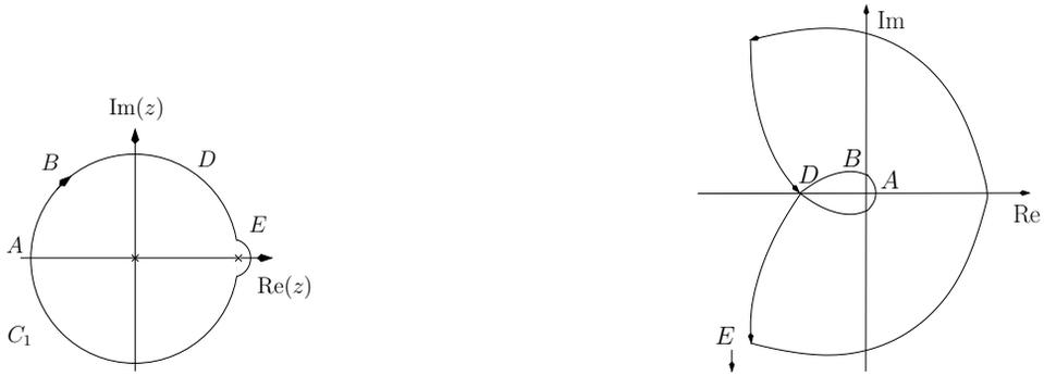
Figure 7.9: Contour  $C_1$  and the corresponding Nyquist plot  $C_4$ , for the system studied in Example 7.2
