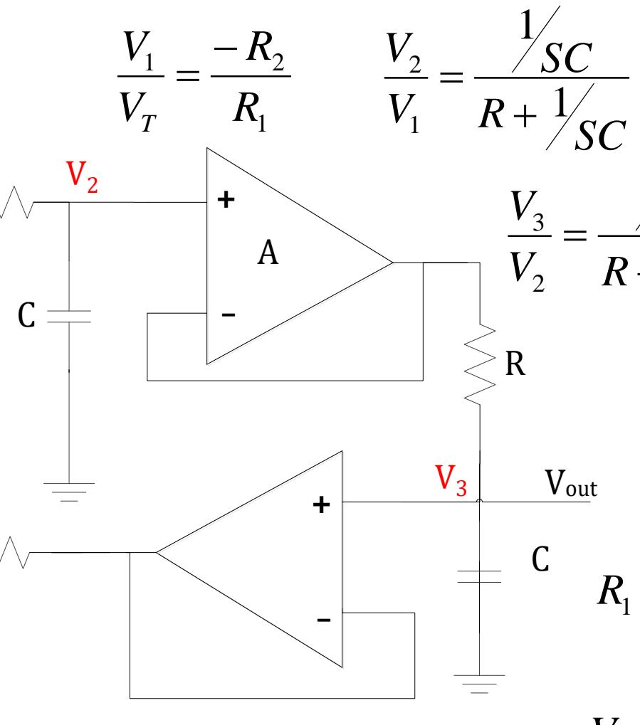
$$T = \frac{V_N}{V_T} = -\frac{R_2}{R_1} \left( \frac{1}{1 + RCS} \right)^4$$
