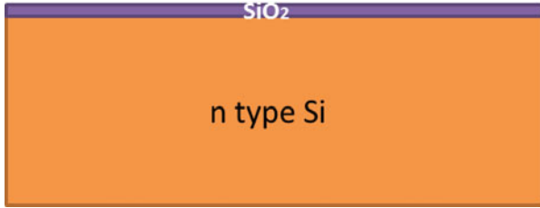
Fig. 5.8 Cross section of step 1: oxidize the Si sample
