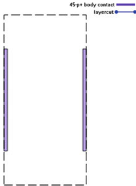
Fig. 7.19 The mask layout of p+ body implant
