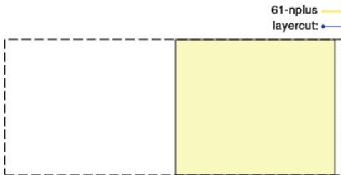
Fig. 6.35 The mask layout of n MOS source/drain implant
