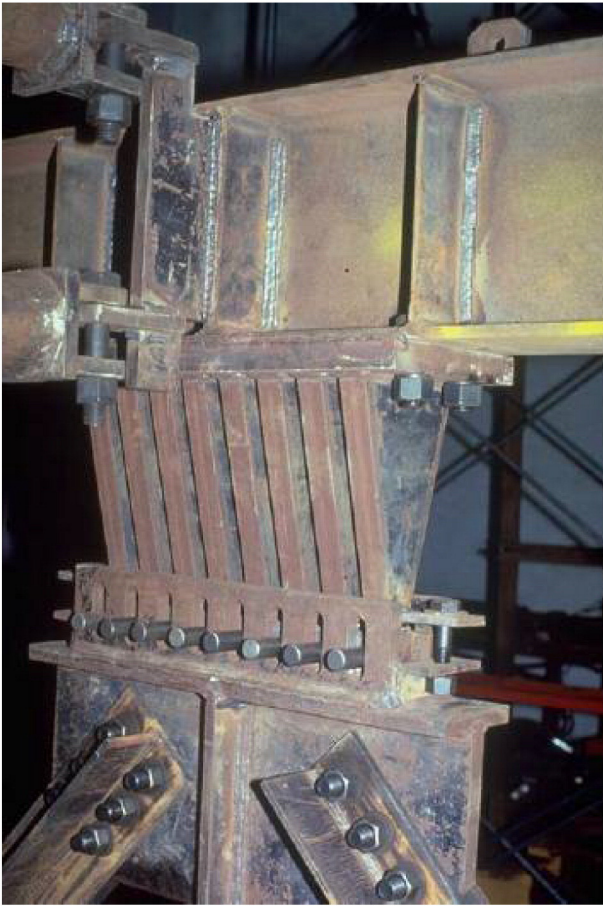
Fig. 1. TADAS device-to-brace connection details [17].
