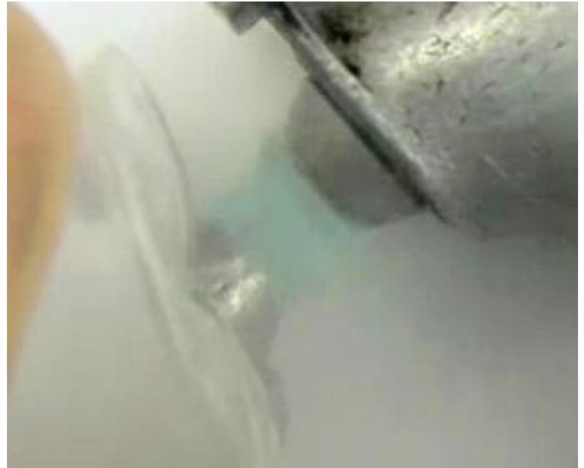
When liquid oxygen is poured from a beaker into a strong magnet, the oxygen is temporarily contained between the magnetic poles owing to its paramagnetism.*
