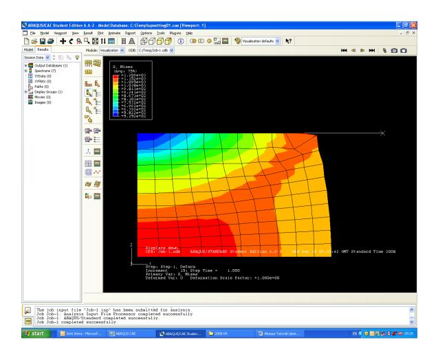
You must use your judgement as to whether the mesh is appropriate (e.g. are the elements small enough), and whether the increment of deformation per step is small enough (specified as -5 in the load module for this example).
